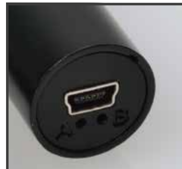
Mini USB port located at the bottom
