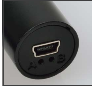
Mini USB port located at the bottom
